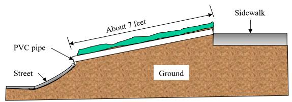
If the line gets clogged with grass clippings and dirt, you can quickly clear it out with a long wire or that drain snake you hardly ever use. If you clear it while the pond is still there, the water will help flush out the line. Be sure the PVC pipe is lined up with the edge of the grass and does not hang over onto the sidewalk. That could be a real toe-stubber for pedestrians—either barefoot or in flip-flips.
